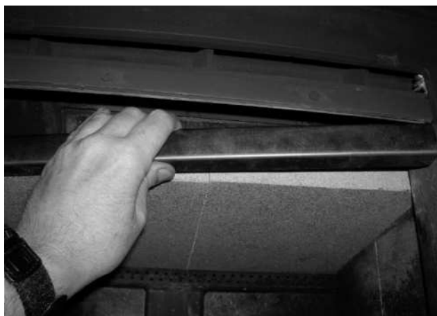
Figure 16 - Removing/Replacing the Baffle for Inspection
