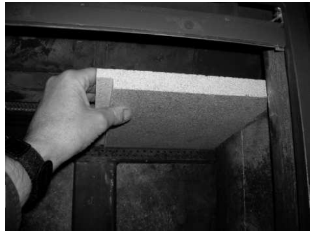
Figure 18 (cont.) - Removing/Replacing the Baffle for Inspection
