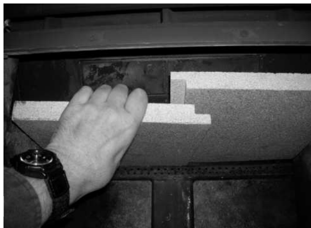
Figure 16 - Removing/Replacing the Baffle for Inspection
